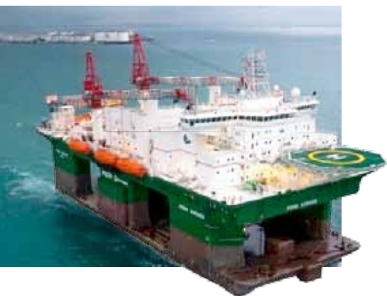
POSH Xanadu is an accommodation rig deployed in the Gulf of Mexico to support Chevron's Big Foot project.
